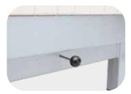
Manual air inlet sliding damper for optimal air supply during firing and reduced cooling times included in the scope of delivery for chamber kilns from 440 liters
