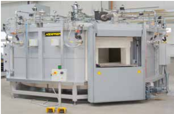
Gas-fired rotary-hearth furnaces for preheating of ceramic moulds up to 1100 °C incl. thermal post combustion for exhaust gas cleaning
