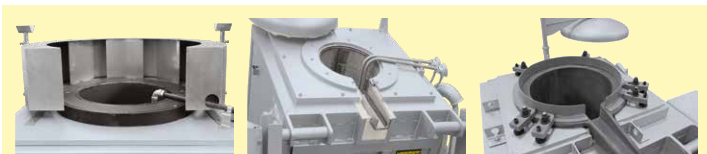
Rim suction ring for connection to customer's exhaust air system
