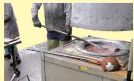
Manual ladling from a bale-out furnace T 80/10
