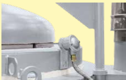
Thermocouple for melt bath control
