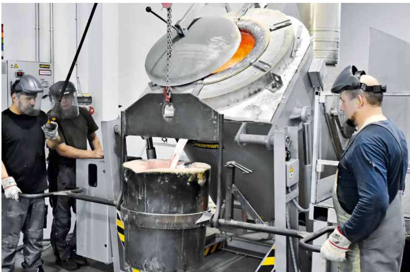
Tilting furnace KB 150/12 in production
