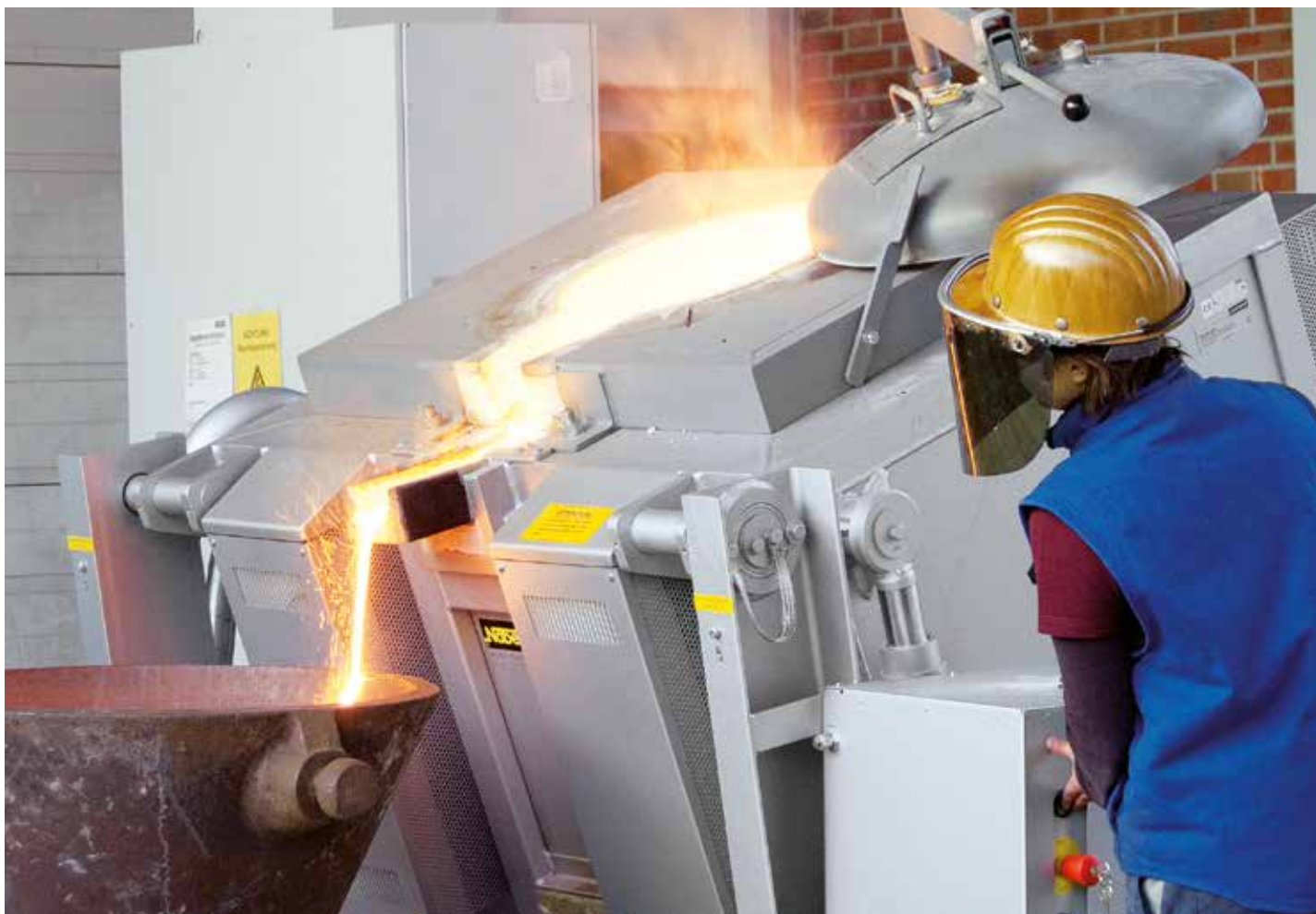
Tilting furnace KC 80/14 during casting
