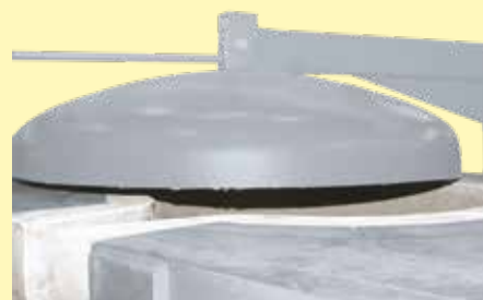
Swing lid with good sealing to collar plate to avoid heat loss over the crucible opening
