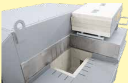
Inlet opening for filling with liquid aluminum
