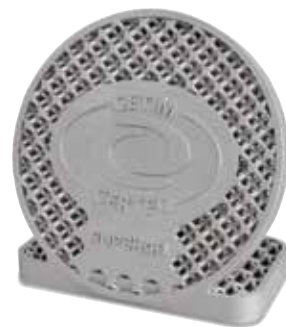
Printed aluminum part, heat treated in model N 250/85 HA (Manufacturer CETIM CERTEC on SUPCHAD platform)
