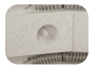
Thermocouple protected in the insulation
