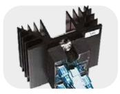
Solid state relays ensure low noise heater operation
