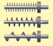
Screw-conveyors with different pitches
