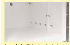
Furnace chamber with air inlet openings for air exchange of more than 6 times per minute
