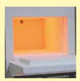
Muffle heated from four sides
