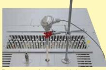
Thermocouple port in the ceiling with tripod
