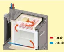
Schematic presentation of air circulation in ashing furnace L 24/11 BO
