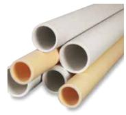
Material Tube outside Ø Max. heat-up ramp Tmax in air<sup>3</sup> Tmax in vacuum operation Gas tight in K/h in °C in °C in mm < 120 unlimited C 530 (Sillimantin)1 1300 not possible no from 120 200 < 120 300 C 610 (Pythagoras)1 1400 1200 yes from 120 200 300 < 120 C 799 (Alsint 99.7 %)1 1800 1400 yes from 120 200 Quartz glass<sup>2</sup> unlimited 1100 950 all yes FeCrAl-Alloy<sup>2</sup> (APM) all unlimited 1300 1100 yes
