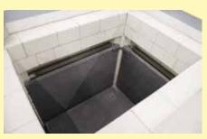
Sides and floor lined with silicon carbide tiles as protection for pit-type furnace S 73/HS
