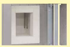
Light-weight refractory bricks and heating elements made from molybdenum disilicide
