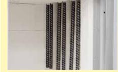
Vertically mounted SiC rods and optional perforated air inlet tubes of the debinding system in a high-temperature furnace
