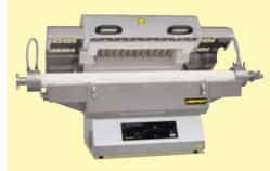
Tube furnace RSH 80/500/13 with gas tight tube and water-cooled flanges
