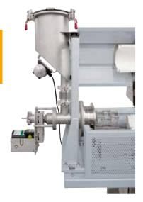
Vibration unit at the charging funnel for improved powder supply
