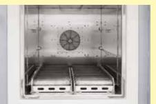
Roller conveyor in furnace chamber
