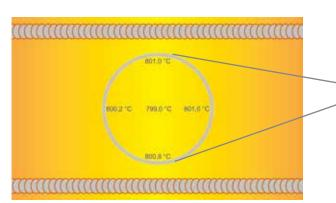
Temperature uniformity, measured in tube furnace RSH 170/750/13
