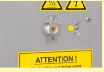
Ashing furnace LV 5/11 with port for thermocouple in the rear wall of furnace
