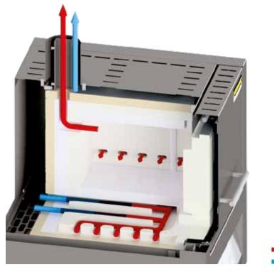
Air inlet and exhaust flow principle in ashing furnaces
