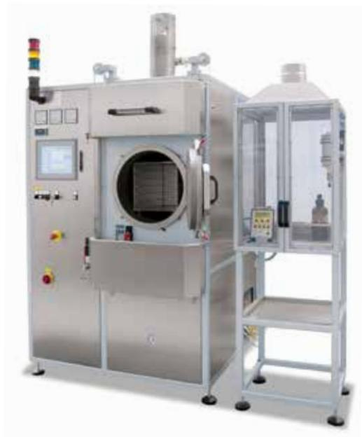
带有酸泵侧柜的NRA 40/02 CDB型甌式炉
