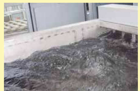
Powerful circulation of quenching medium
