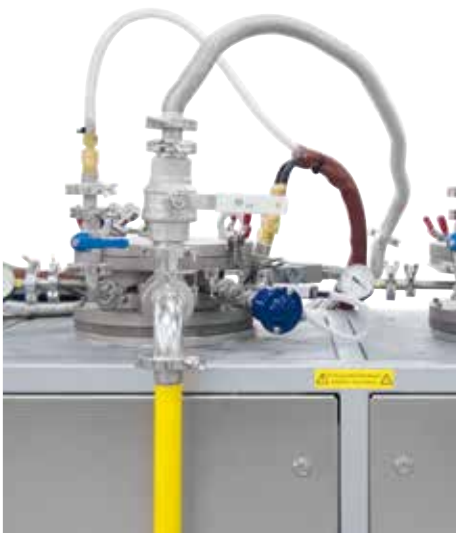
Exchangeable retorts with supply and measuring lines
