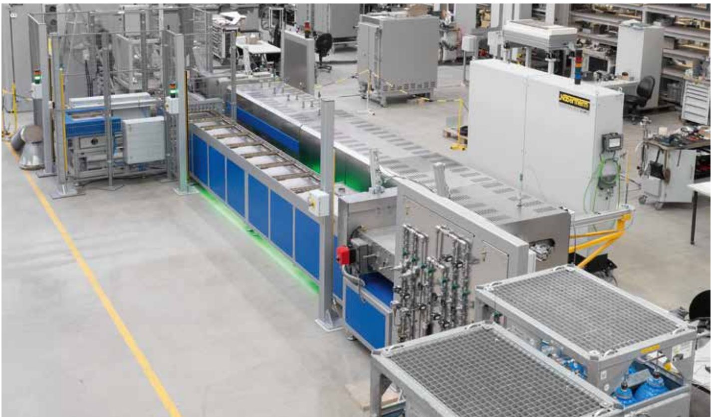
Pusher-type furnace system D 520/2600/55-04 S to sinter teflon coatings under protective atmosphere
