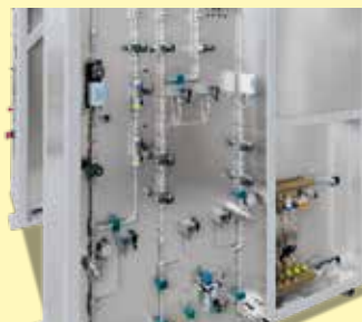
Gas management system at bottom loading retort furnace LBR 300/11 H 2
