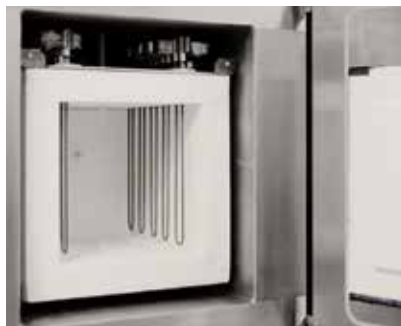
Molybdenumdisilicide heater and fiber insulation
