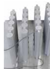
Titanium rods after heat treatment in NR 50/11 in argon atmosphere
