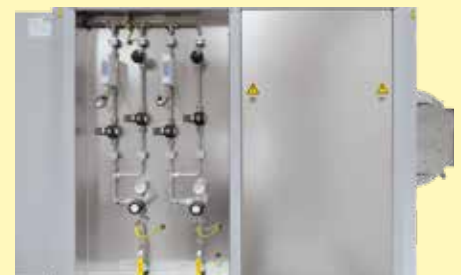
Gas supply system with mass flow controller
