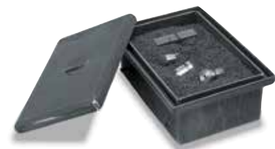
Annealing box with lid and granulate
