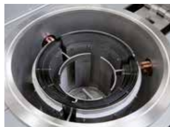
Cylindrical retort with tungsten heating
