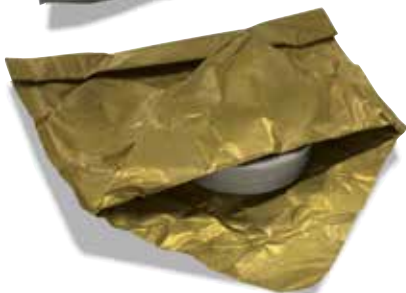
Workpieces in foil heat treating
