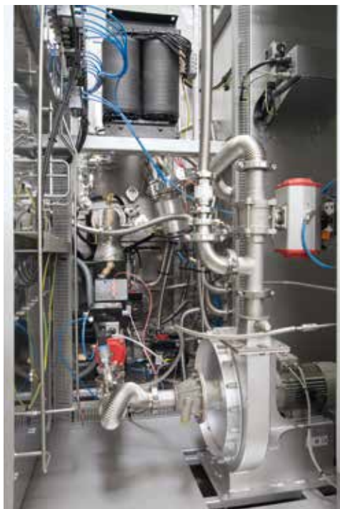
Rapid gas cooling, cold-wall retort furnace VHT 8/16-MO
