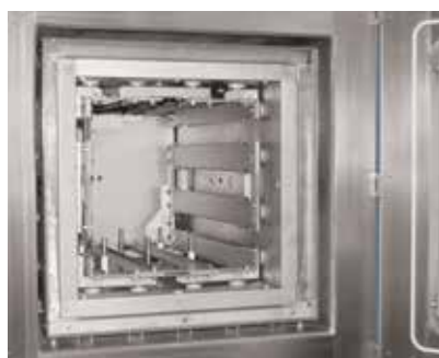
Molybdenum or tungsten heating chamber
