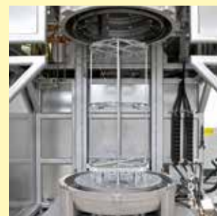
Retort furnace LBVHT 540/16-MO H 2 with measuring frame
