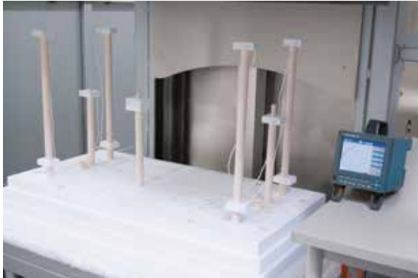
Measurement set-up in a high-temperature furnace
