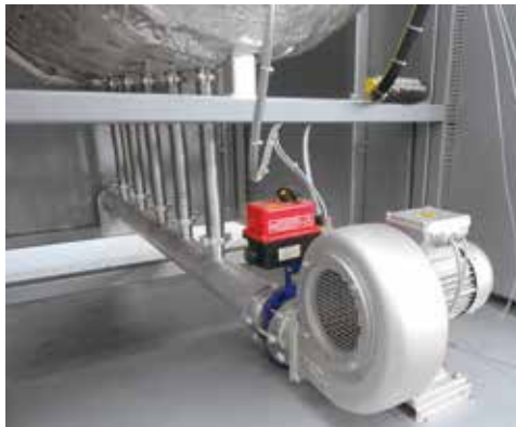
Fan cooling, hot-wall retort furnace NRA 400/03
