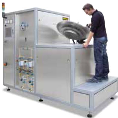
Retort furnace SVHT 9/24-W with tungsten heating
