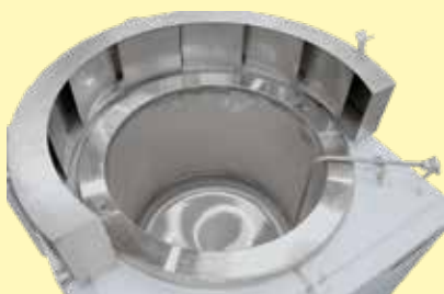
Salt-bath furnace TS 90/80 with a salt bath thermocouple for heat treatment of steel
