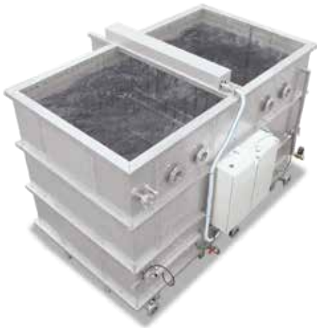
Water quench tank WAB 24000 with forced circulation
