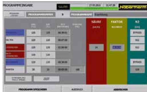
Heating program input screen of the CDB furnace
