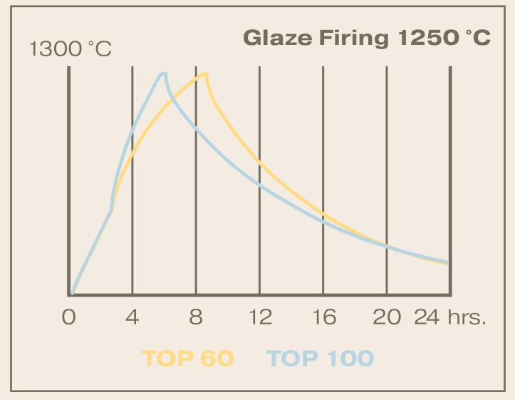
Example curve of a glaze firing
