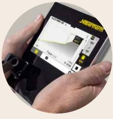
Controller with touch operation C540 (10 programs with each 20 segments)
