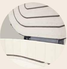
Interior with bottom side ring heating on fusing furnaces F 75 – F 220
