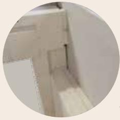
Multi-layer refractory insulation with light-weight refractory bricks
