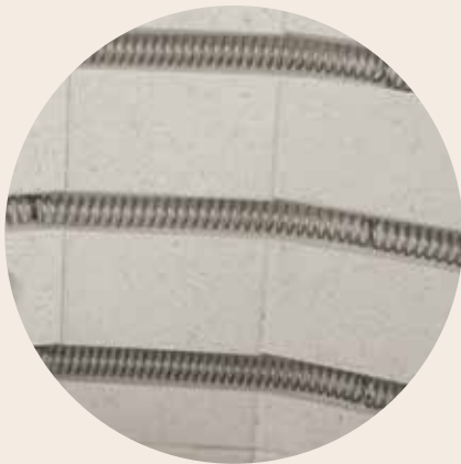
All-round heating elements, protected in grooves made of APM wires
