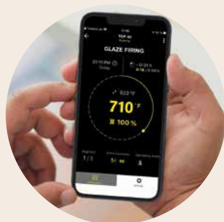
Display of program progress for each kiln
