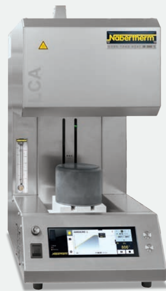
配备退火罩套装的组合炉LCA 04/13 LB
