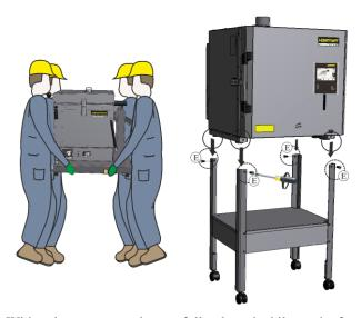
With at least two people, carefully place the kiln on the frame and make sure that it sits properly. Then screw the kiln onto the frame at the positions illustrated (E).
