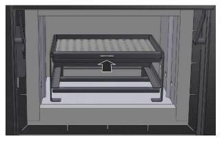
A charging handle is supplied to insert and remove the trays which may be hot; hook this handle into the notch at the front of the tray.
