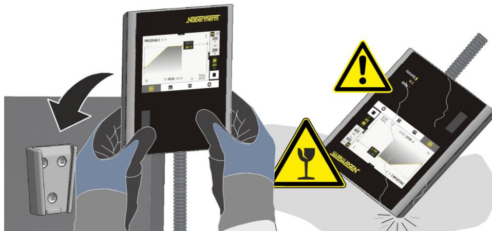
Fig. 19: Place the controller in the holder on the furnace (similar to the picture)
