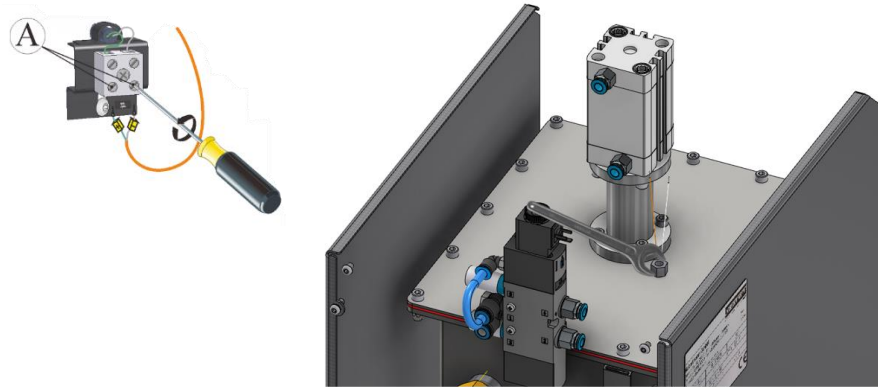
Fig. 42: Dismantling the thermocouple (similar to picture)
