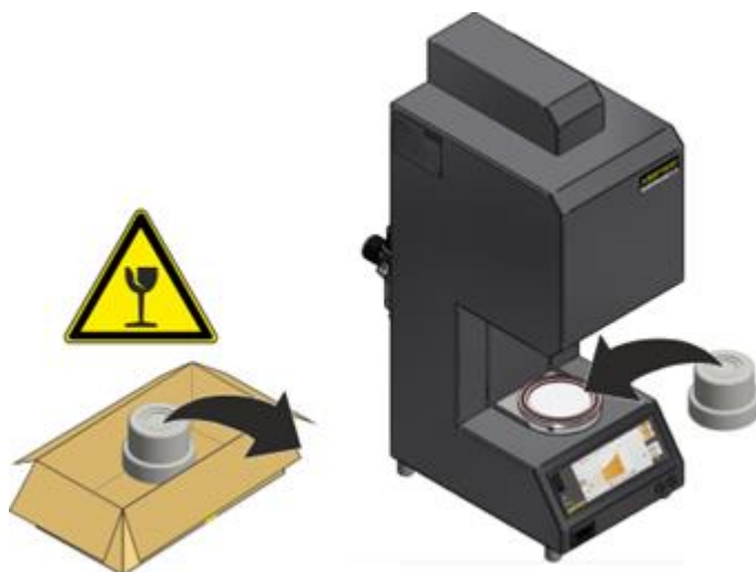
Fig. 15: Placing the insulation on the lift bottom (similar to picture)
