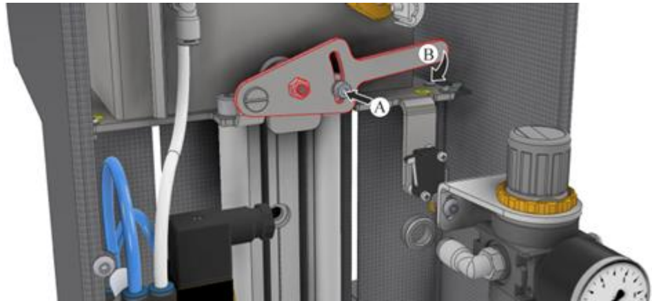
Fig. 29: Undoing the belt tensioner (similar to picture)
