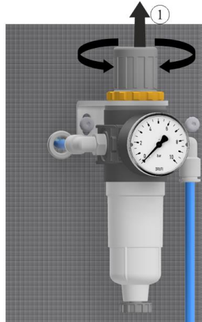
Fig. 12: Adjusting the pressure at the compressed air-maintenance unit (similar to picture)
