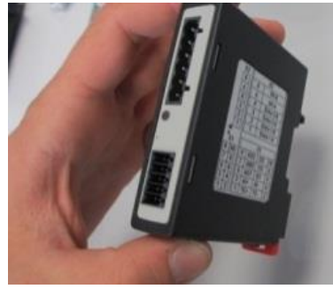
Fig. 10: Removing the controller module - part 2 (similar to picture)
