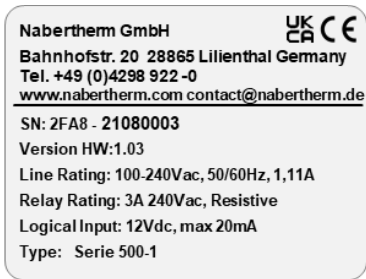
Fig. 7: Example (type plate of the control unit)
