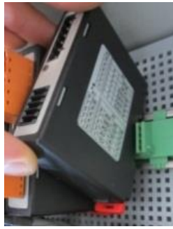
Fig. 10: Removing the controller module - part 2 (similar to picture)
