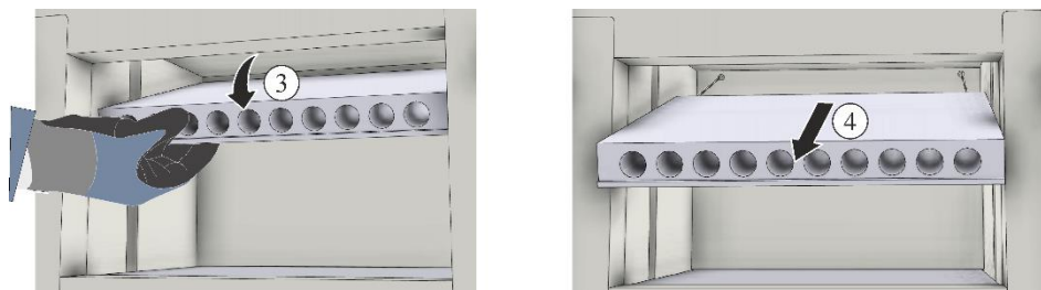
Fig. 16: Dismantling the upper heating plate (similar to picture)
