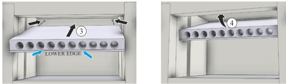
Fig. 68: Installing the overhead heating (pay attention to the lower edge) (similar to picture).
