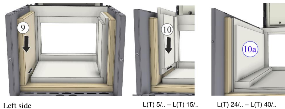
Fig. 49: Installing the side insulating panel and insulation (similar to picture)
