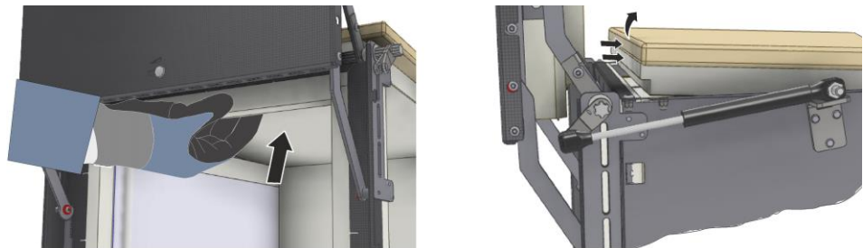
Fig. 72: Carefully push the roof insulation upwards (LT 60/..) (similar to picture)
