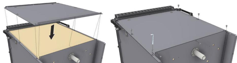
Fig. 74: Installing the furnace ceiling (similar to picture)
