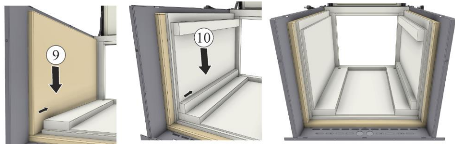
Fig. 59: Installing the side insulating panel and insulation (similar to picture)
