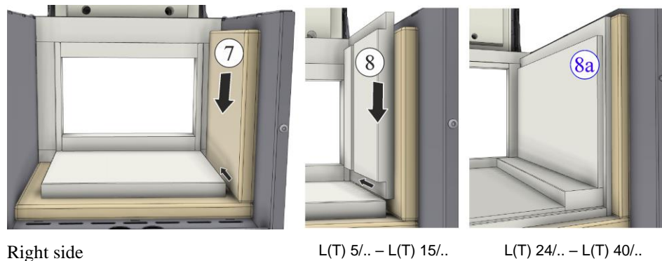
Fig. 48: Installing the side insulating panel and insulation (similar to picture)
