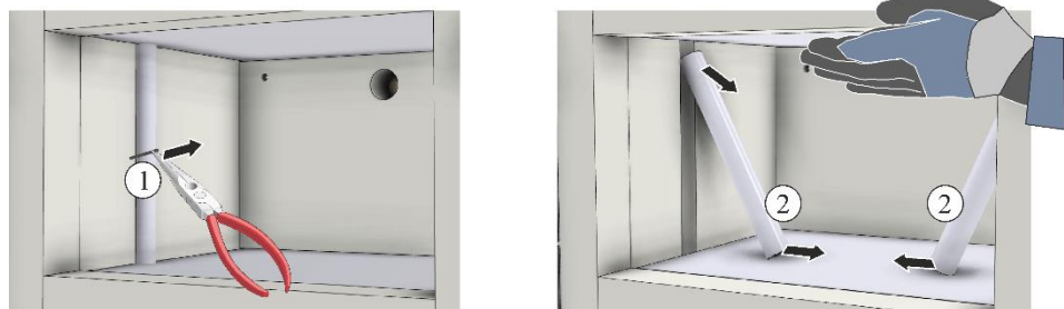
Fig. 15: Dismantling the heating plate supports (similar to picture)
