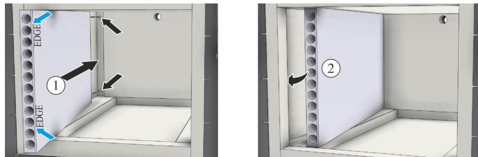
Fig. 70: Fitting the side heating plates (similar to picture)
