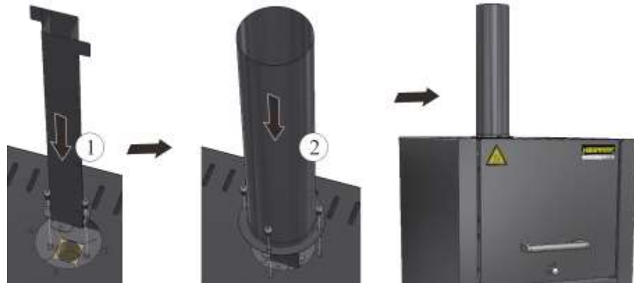
Fig. 24: Installation of an exhaust gas pipe on LV(T) models (similar to picture)
