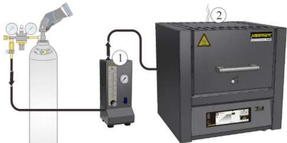
Fig. 51: Connection to the gas supply system (similar to picture)
