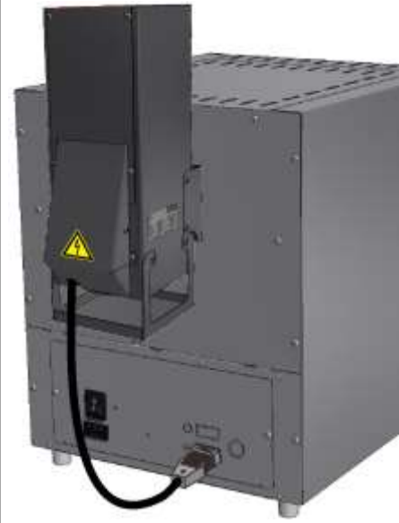
Catalytic converter with fan for removal of organic components from the exhaust air. Organic components are catalytically oxidized at about 600 °C, broken into carbon dioxide and water vapour. Irritating odors are thus largely eliminated. The B510 – P580 controllers can be used to switch the catalytic converter automatically (not for models L(T) 15..., L 1/12, LE 1/11, LE 2/11).*
