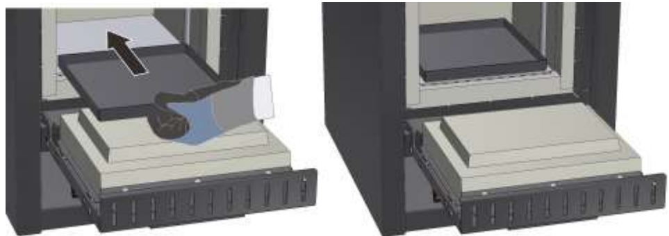
Fig. 36: Example: Careful depositing of the catch basin (similar to picture)
