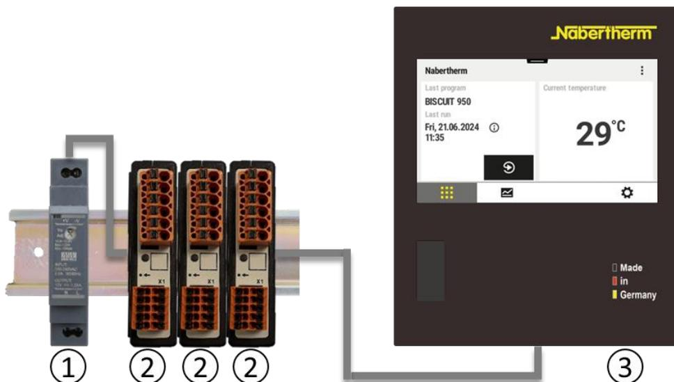
Voltage supply (1) and control modules (2) are located in the switchgear; the operating and display unit (3) can be installed in the front or side of the switchgear or in the front of the furnace. The control modules (2) are linked via a pluggable backplane bus connector.
