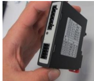
Fig. 12: Removing the controller module - part 2 (similar to picture)
